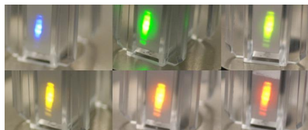
Figure 1. UC fluorescent labels developed by the authors demonstrating a wide range of possible emission colours when excited at 980nm ( 0.2 \text{ W/cm}^2 ) (adapted from [1]).
