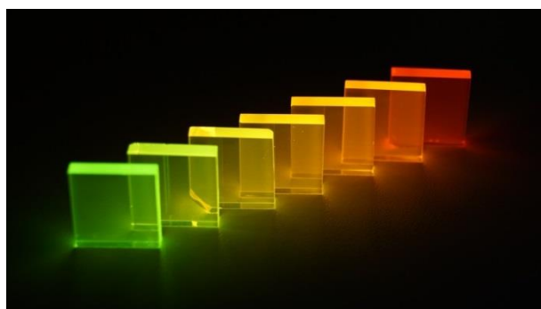
Figure 1. \text{Eu}^{3+} and \text{Tb}^{3+} single- and double-doped borate glasses under ultraviolet excitation.
