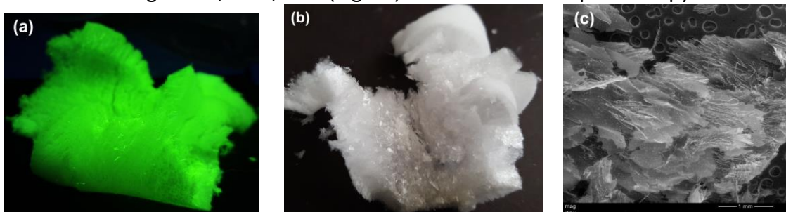
Figure 1. The prepared poly(N-Isopropylacrylamide)- \text{Tb}^{3+} aerogel (a) under UV excitation, (b) in ambient lighting conditions, (c) SEM image of the aerogel
