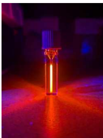
Figure 1: Picture of a luminescent curium complex in solution.
