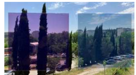
Figure 1: Laminated photochromic films of 28 x 28 cm under direct sunlight irradiation.
